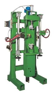
Flame-processing in combination with mechanical tools allows to punch holes into the hot glass, which is necessary for light-sources, mixing equipment etc.
