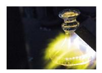
The burning-off unit has been designed for removing the top or cap of blown articles. Burning-off the top leaves the rim slightly thicker than the wall, and - given this visual implication - it is generally used for glasses with a safety rim and for glass items which incorporate this rim into their design.
